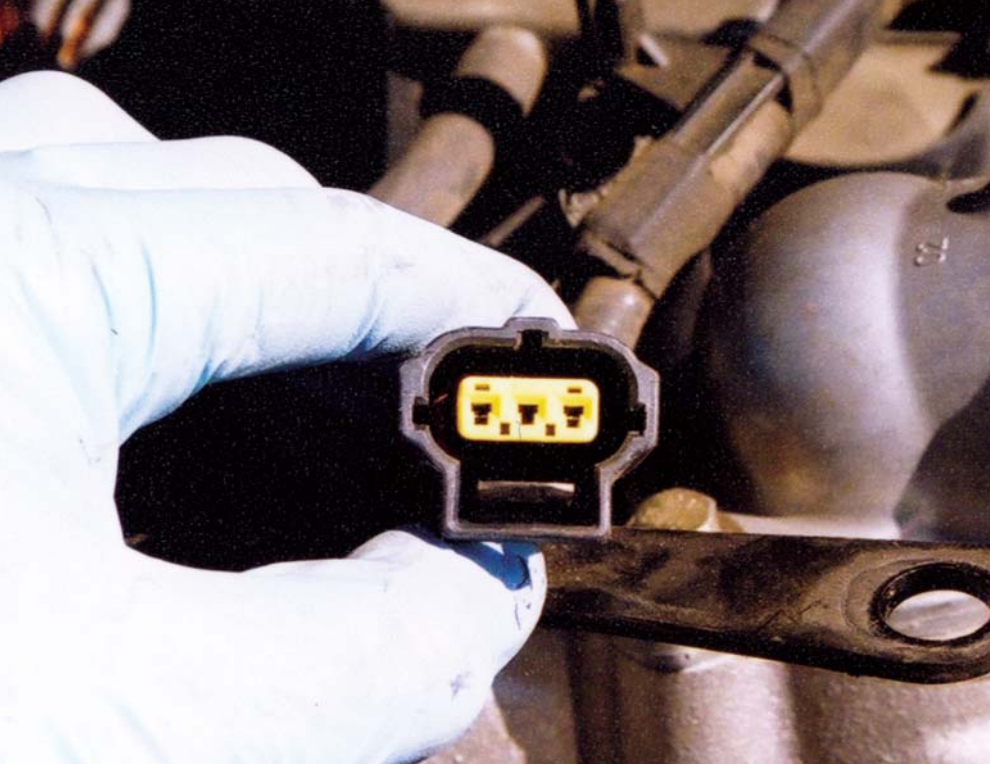
Often the connectors are different on replacement alternators. Some alternators have a "D" shaped connector, instead of the rectangle shape as shown, which will not fit the Police Interceptors.
