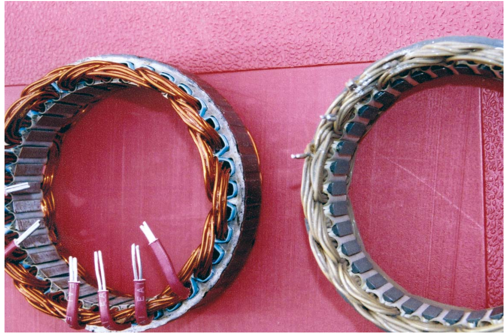
Heavier gauge wiring on Quality Power's alternators (left) allow it to produce more amperage than the stock Ford alternator (right).
