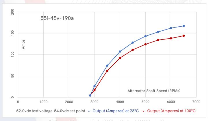
Testing conditions completed at 23°C ambient and 100°C in a hot box.
