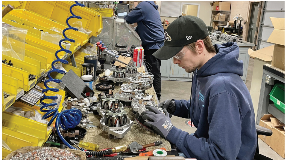
Aaron Ransavage, an assembly and test technician with American Power Systems, assembles alternators in APS’ manufacturing facility headquartered in downtown Davenport. CREDIT AMERICAN POWER SYSTEMS
